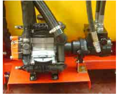
Pump 120 l/min + hydromotor
